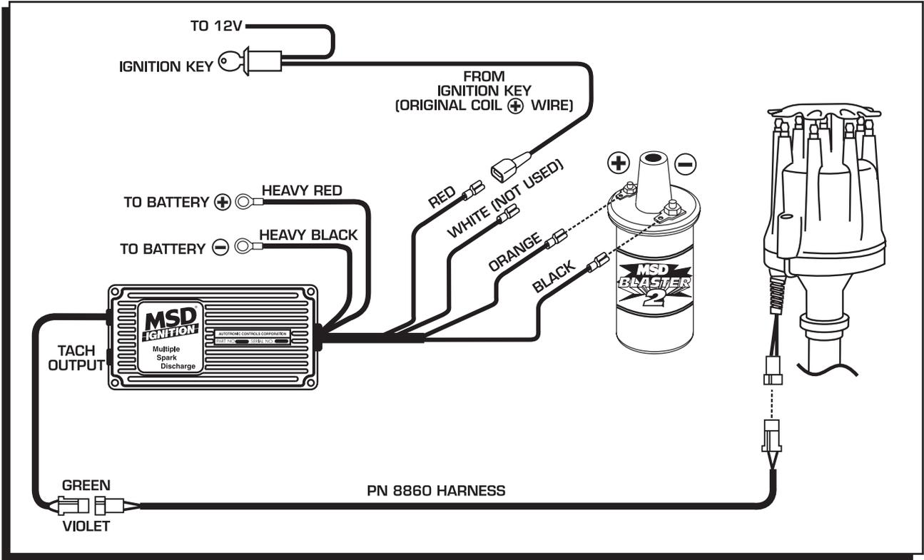
Figure 12 Wiring to an MSD 6-Series Ignition Control.
