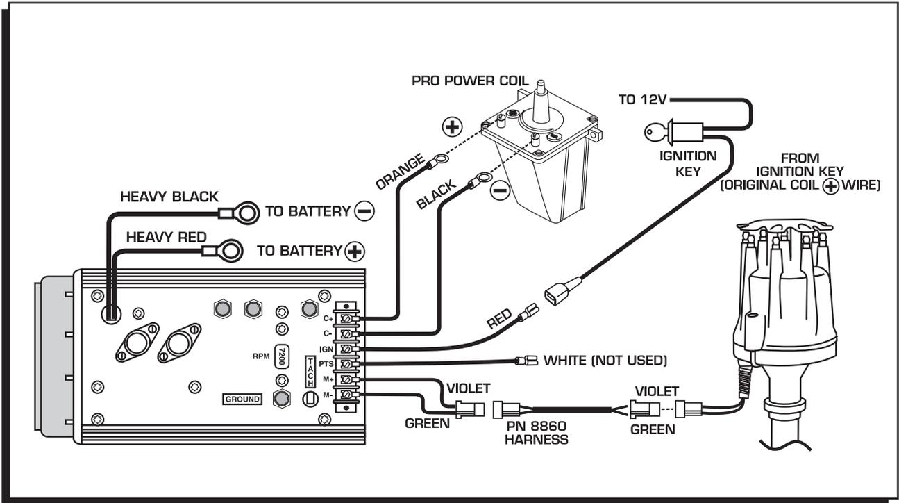
Figure 13 Wiring to an MSD 7-Series Ignition Control.
