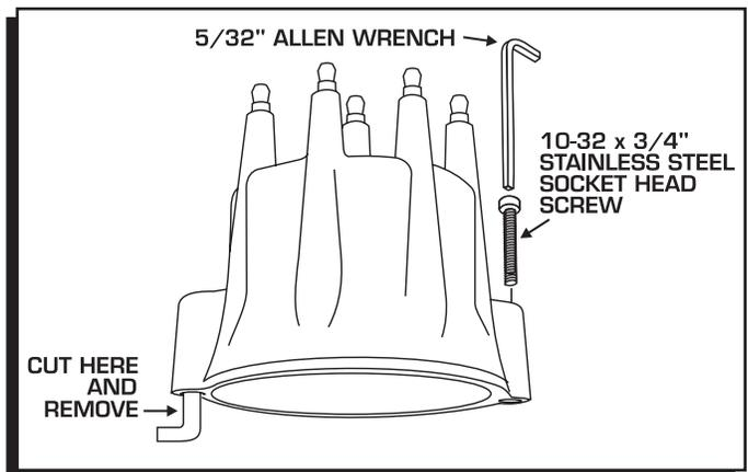
Figure 10 Optional Installation by Bolting Cap Down.
