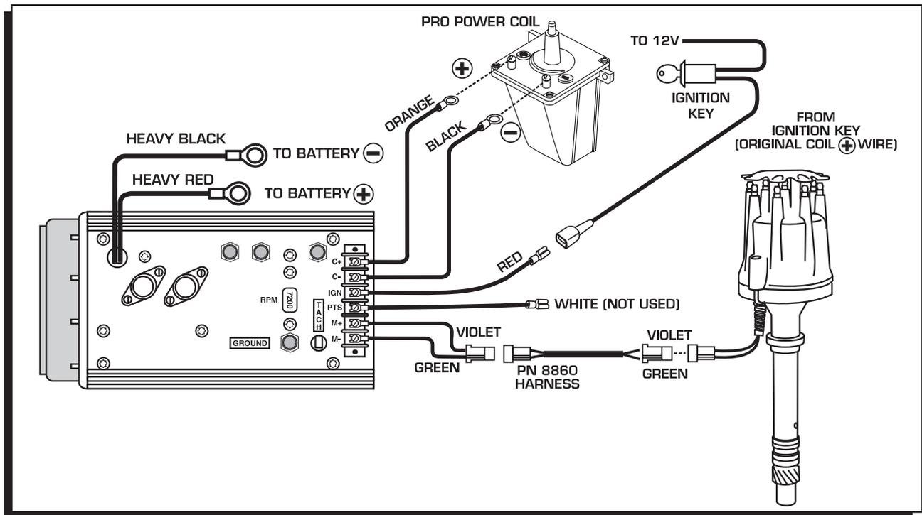
Figure 14 Wiring to an MSD 7-Series Ignition Control.
